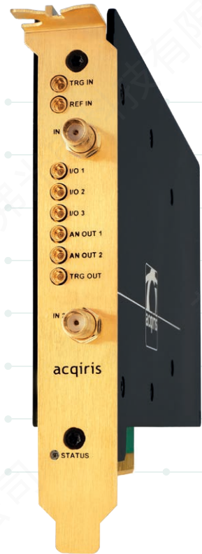
Figure 6. The SA220P is a fully shielded PCIe Card maximizing both ESD and EMI protection.
