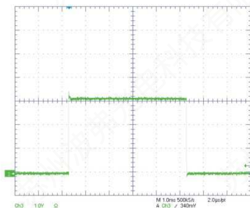
Figure: Current monitor output, scale: 100A/Div
