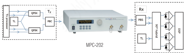
Fig. 1 SOP tracking speed and recovery time tests in a coherent detection system. The General Photonics MPC-202 can be used for these tests.
